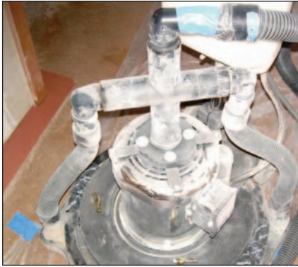
A 110-volt multi-surface machine can be used in the polishing and grinding process.
