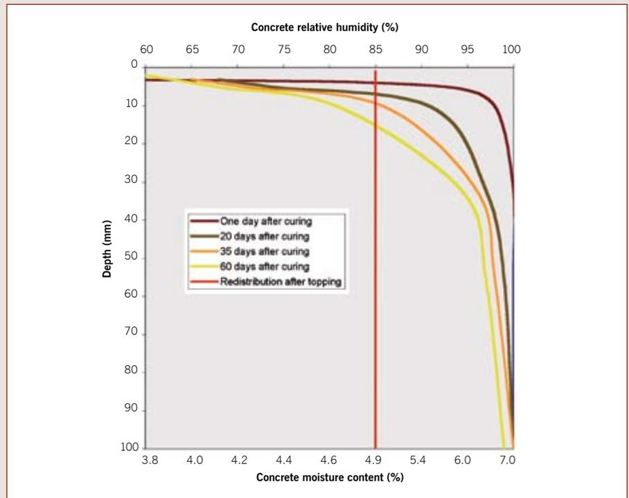
Figure 1: Moisture profiles in a drying concrete slab.
