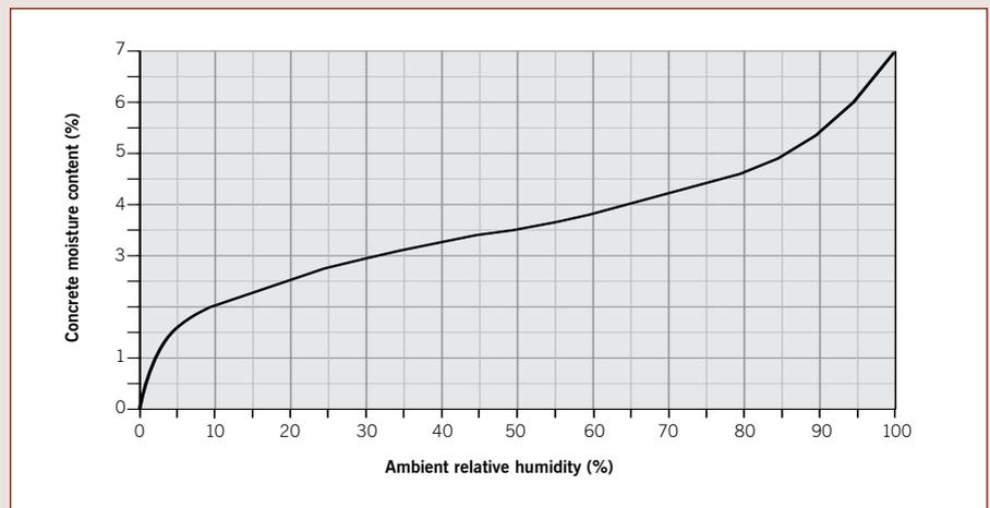
Figure 2: Sorption curve for concrete.
